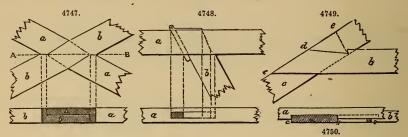
Figs. 4749, 4750, show the mode of notching a collar-beam tie into the side of a rafter by a dovetailed joint. The general remark as to dovetailed joints applies with especial force to this example.
